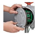
With the dual-sealed Separate Terminal **Chamber (STC),** installation wiring can be terminated and fuses can be replaced without exposing the internal control components to hostile environmental conditions.
